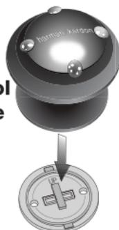
Push the knob down onto the base, and turn clockwise to lock it into place. The knob can be removed by turning the bottom counterclockwise.
